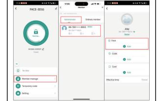
When adding a face, the camera flashes quickly, the indicator light turns green, and you can hear "Di" voice, indicating added successfully, click "Done"
